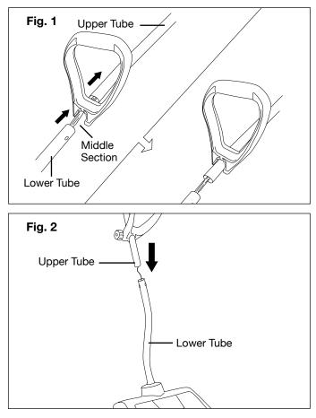
**2.** After sliding upper tube inside the lower tube (Fig. 2), line up the screw holes on each tube.
