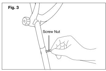
**3.** Insert the screw nut through the aligned holes in the upper and lower tubes and secure other end with the knob (Fig. 3 and 4).
